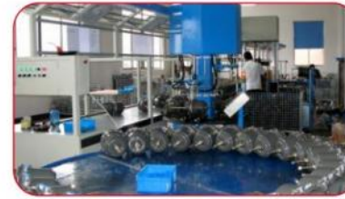
Brake chamber assembly line
